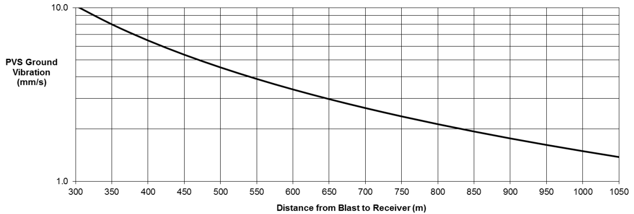
Figure 2 Peak Particle Velocity Ground Vibration (5% Exceedance) for an MIC of 48 kg
